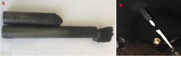
Fig. 2. (a) Anode consumption and slag formation, (b) reactor inner surface after experimental studies.
